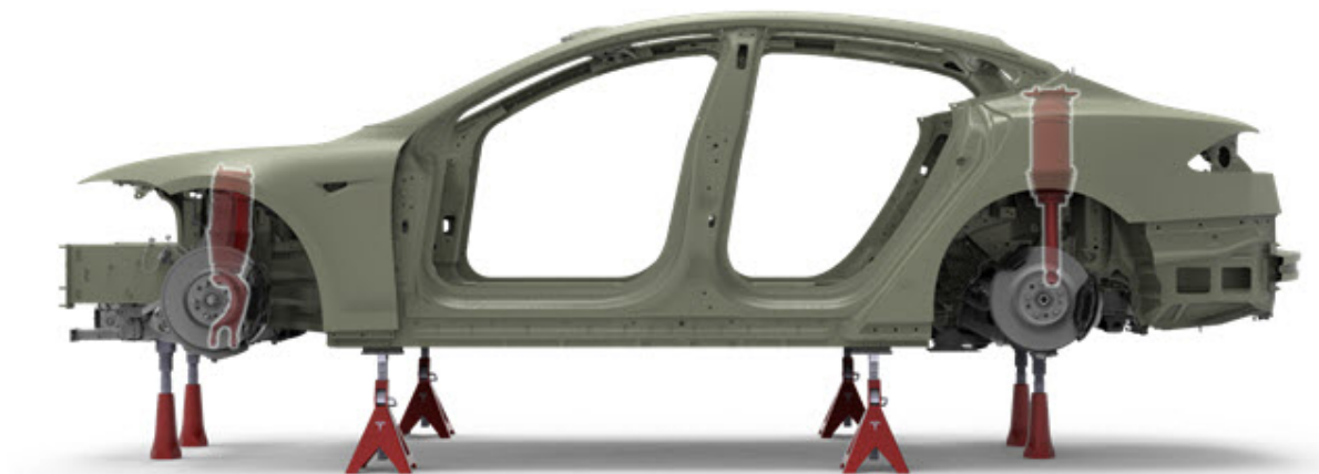
Figure 1. Example of vehicle setup with jacks and spring assemblies highlighted in red
