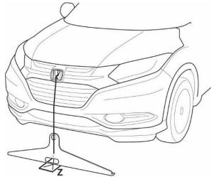
4. With the cord or string centered with the center line of the centering stand, make a new mark Z1 using the listed distance in the service information.
