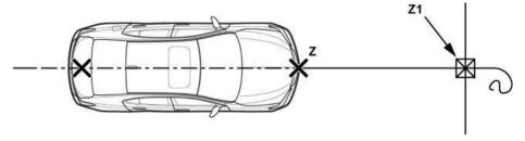
5. The target set up you just completed should match the one in the aiming procedure. You are now ready to set up either the radar or camera target stand.
