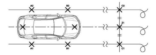
Some models, like the Accord and Civic, will require an additional reference mark as the radar is mounted to the side. This mark can be simply made on the tape placed in step 12. Refer to the aiming procedure for additional information.
