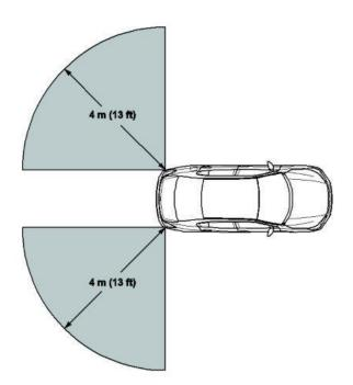
Radar, FCW/LDW Camera, or Multipurpose Camera Aiming
