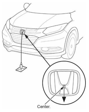
3. Place the centerline of the centering stand from Alignment Set (T/N 07AAJ-STKA210) on mark Z, then run the cord or string through it.
