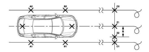
The procedure mentioned can also be used when setting up the LaneWatch camera aiming. Instead of in front of the vehicle, use the procedure to set up the reference marks behind the vehicle.
