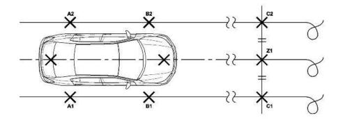
1. Place the centering stand from Alignment Set (T/N 07AAJ-STKA210), at the center of the right-rear wheel. Extend the pointer as needed or as much as possible so it reaches the edge of the center cap.
