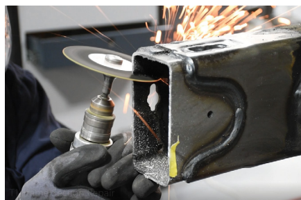
▶ A technician removes the remaining portions of the existing frame end.
