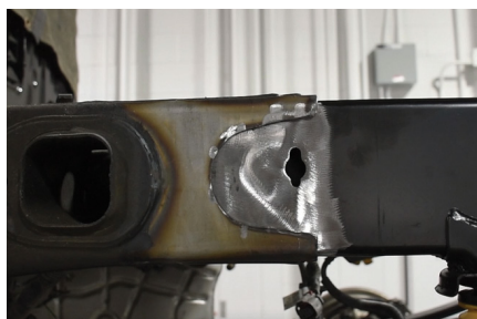
▶ The new GM-engineered frame section mates precisely with the existing frame end.
